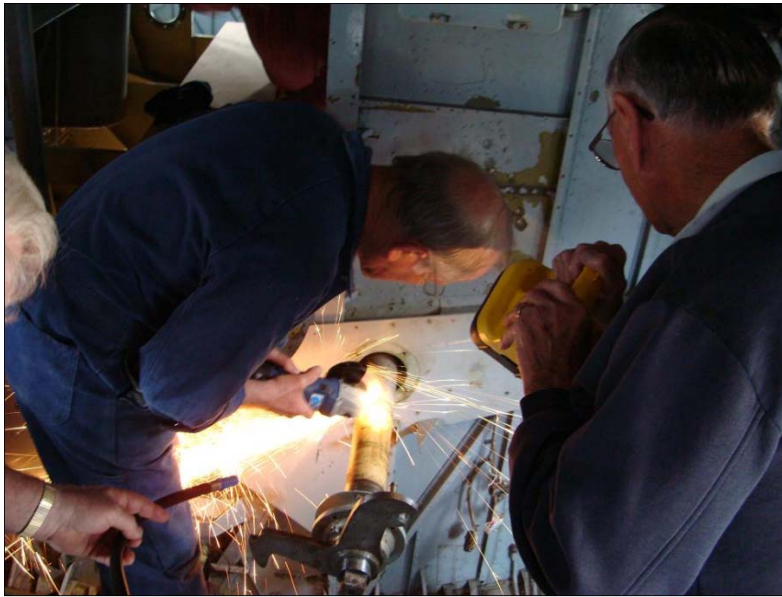
Bruce Richardson works to cut the bomb-bay door actuating shaft, assisted by John Goldsborough (L) and Len Linfoot (R). (Photo: P. Parrague)
